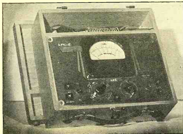
Figure 1: The set tester, with its cover removed to show the control panel, including meter, the master selector switch, the zero adjuster, and other controls. At the top is a compartment for the test leads.
